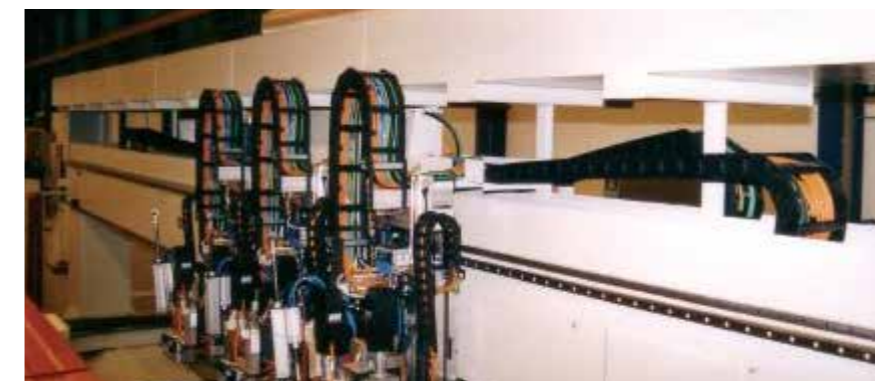
Woodworking machines with e-chains® and chainflex® cables
