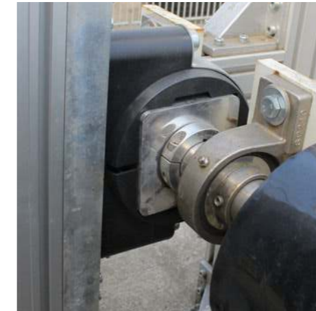
The ESQM 2.0 was subjected to an intensive wear test on the outdoor test rig. The test comprised a total of 18,900 cycles with a constant test load of 7.5kN.
