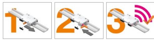
Simple bearing liner replacement
