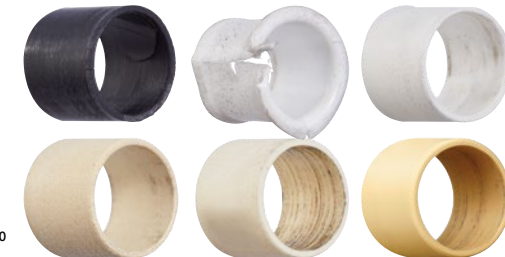
Wear, rotating p= 20MPa; v= 0.01m/s, VA
