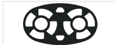
Steel inner plates absorb the force of the fixed stop dogs of the plastic outer links.
