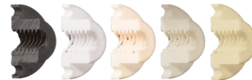
Wear test: drive nut F= 129N; l= 370mm; n= 290rpm
