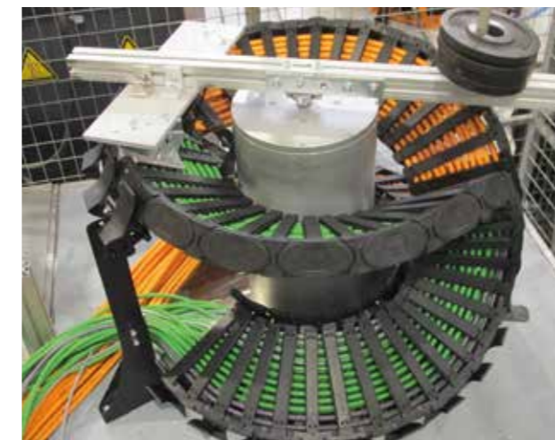
Rotary movement tests in very demanding chain applications using igus® twisterchain®
