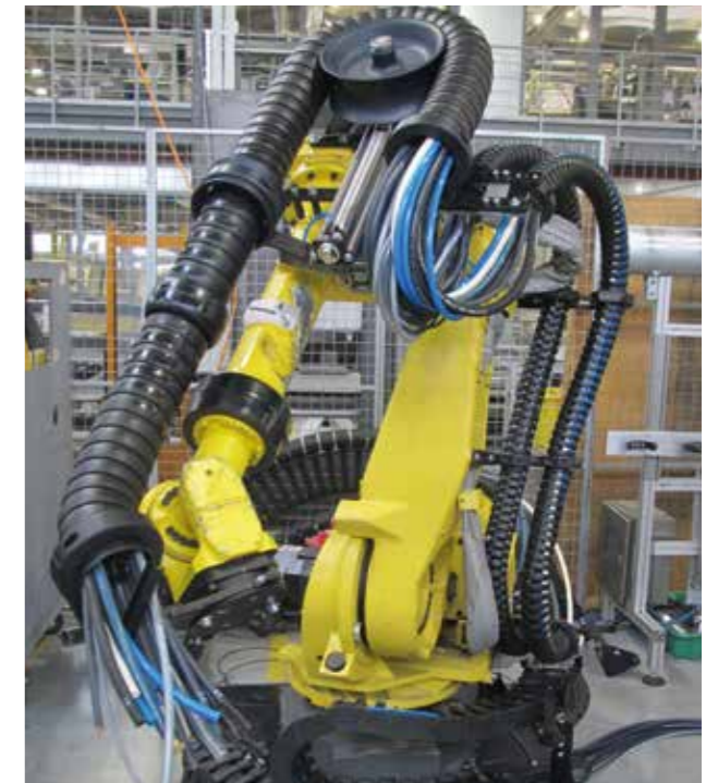
Test for complex movements by simulating multi-axis applications on robots
