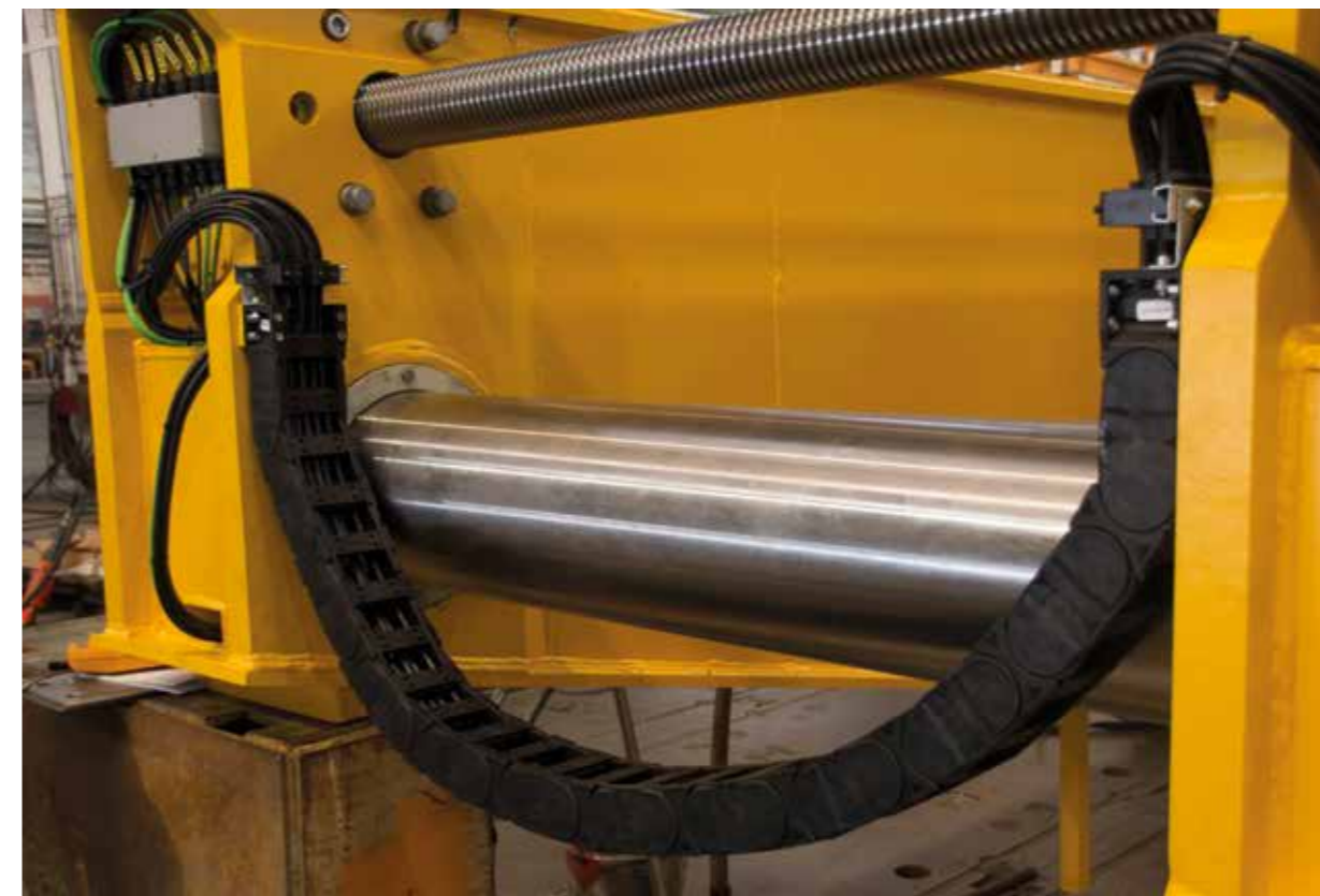
chainflex® CF891 in an adjustment device for a process crane
