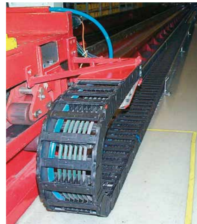
chainflex® CF5/CF6 for storage retrieval unit: Long travel in longitudinal axis. e-chain®: Series E4/00 with igus® guide trough made of steel
