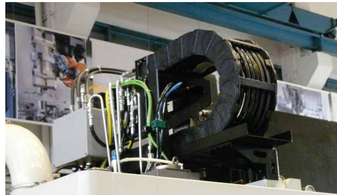
chainflex® CF880 in a short travel application
