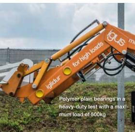
Possibly the world's largest test database has been created from over 15,000 tests per year. It enables us to always select the right product for your specific application. Individual tests can also be performed for your industry.
