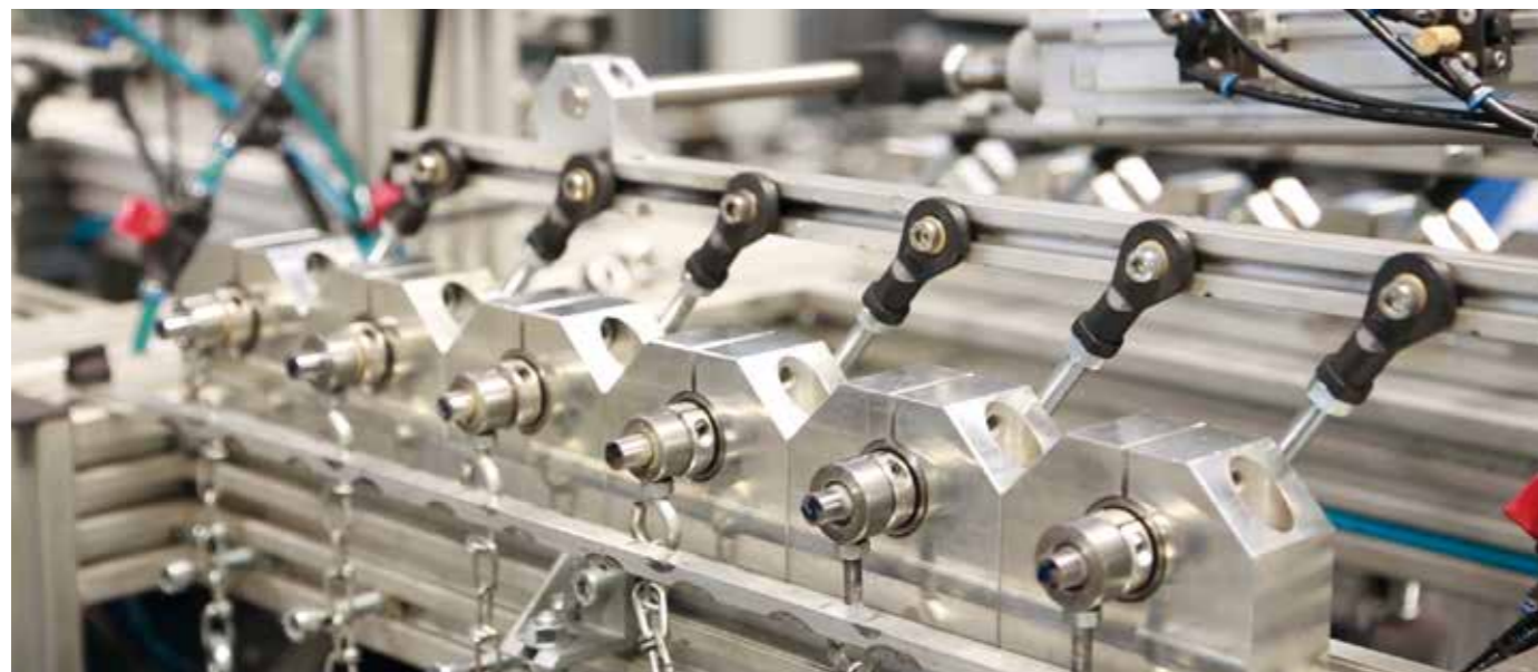
Picture 01: igus® test lab: More than 13,000 tribological tests (friction and wear) each year in 300 test rigs in the industry's largest laboratory (3,800m²). View inside igubal® test rigs.
