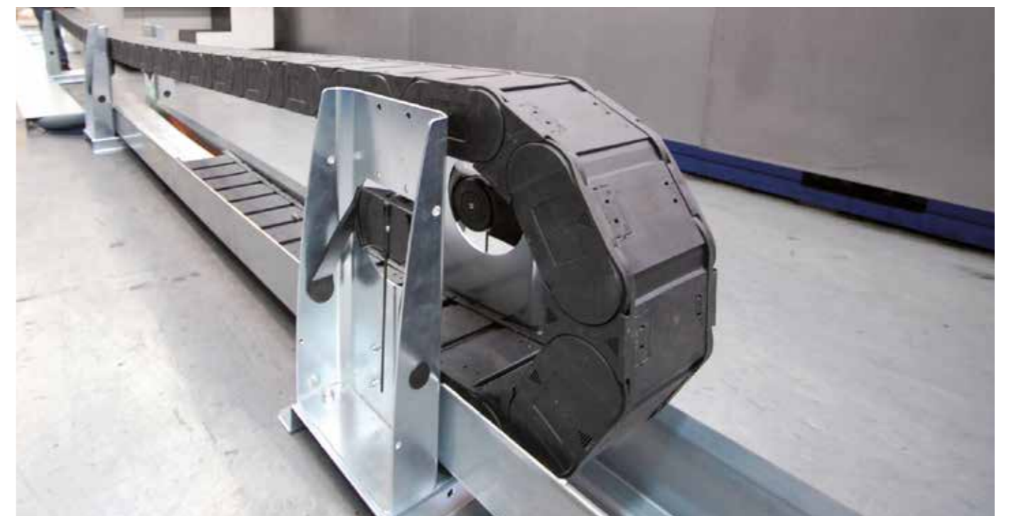
guidelok - swarf-proof and unsupported over long travels, more cost-effective than most steel chains or complex gliding systems
