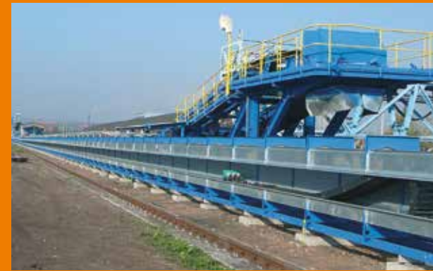
Extremely long travels with rol e-chains® (here 615m)
