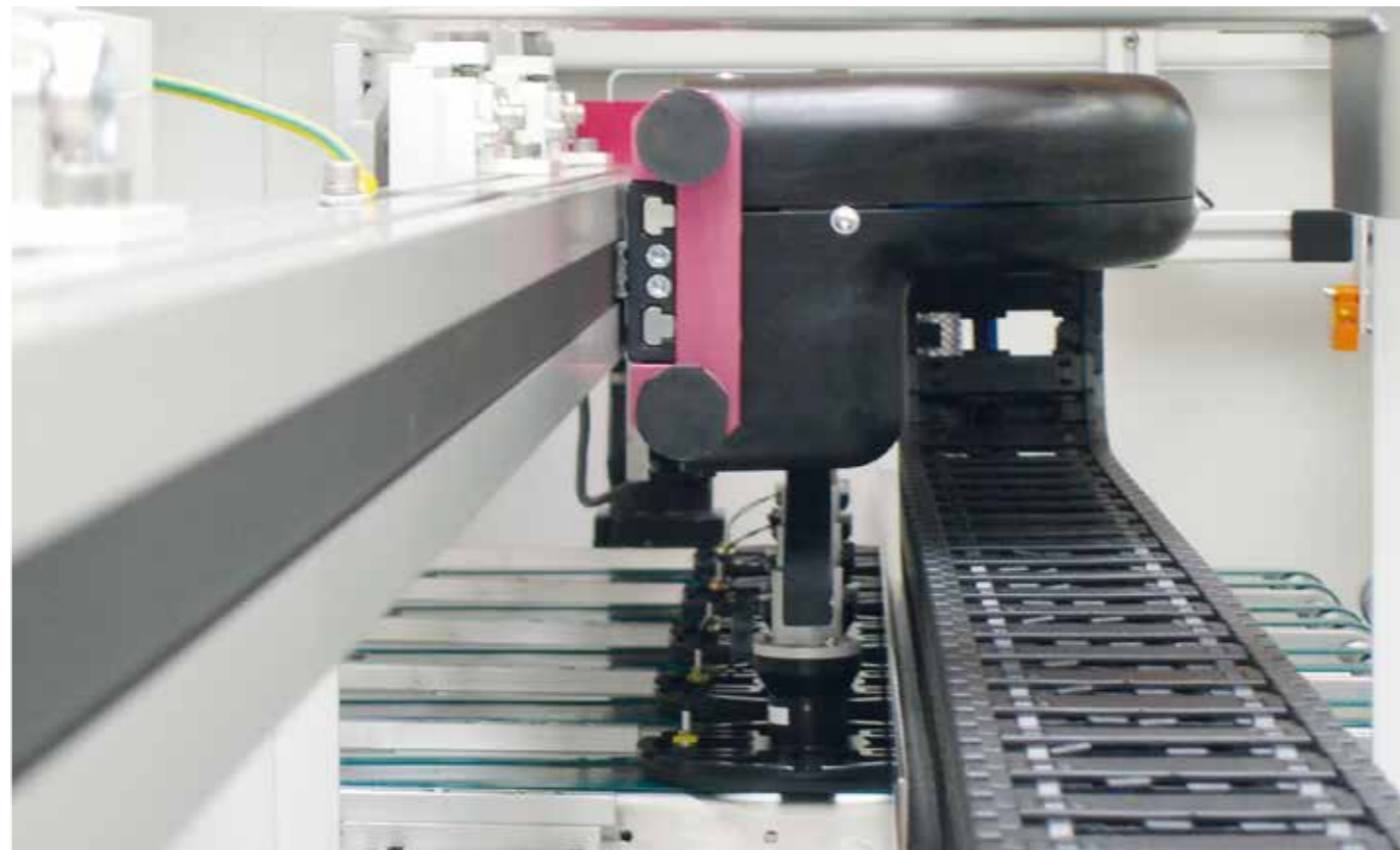
e-chain® from the E6 range accelerates work processes in the wafer-handling application in chip production
