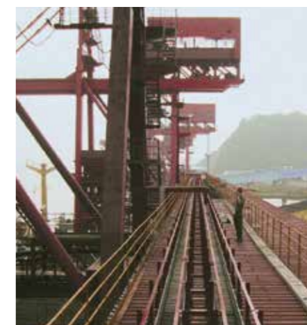
rol e-chain® on a coal unloading system with fire protection regulations - travel 190m, fill weight 8kg/m, travel speed 0.5m/s
