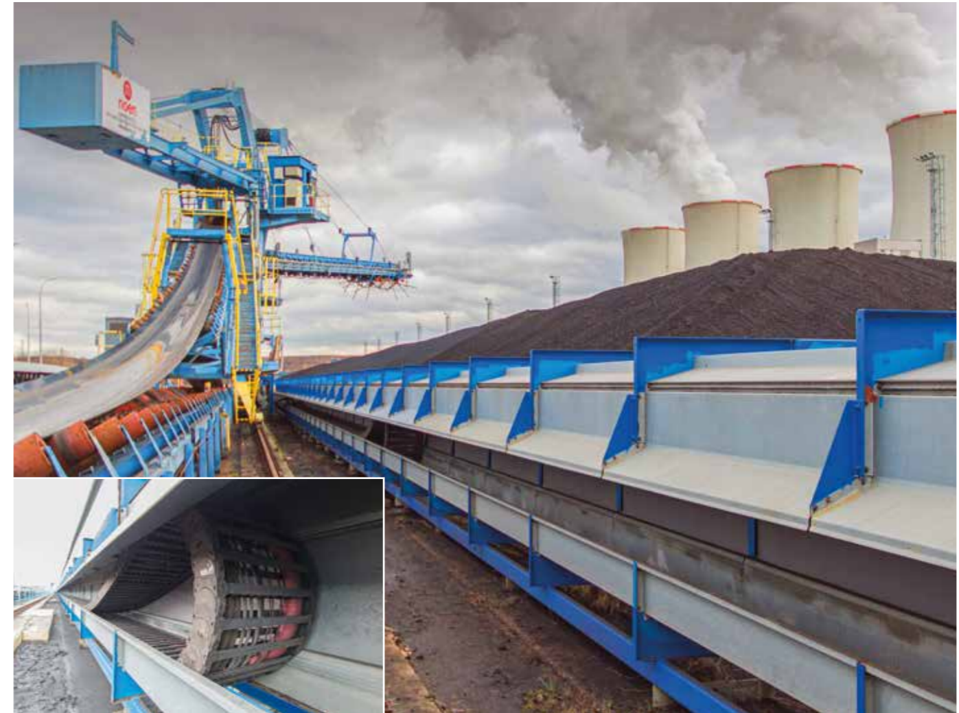
World record application - 615m travel in operation since 2008 without failure. In addition to the motor, control and data cables, a water hose is routed in the e-chain® of the E4/4HD system (shown right in the e-chain®)
