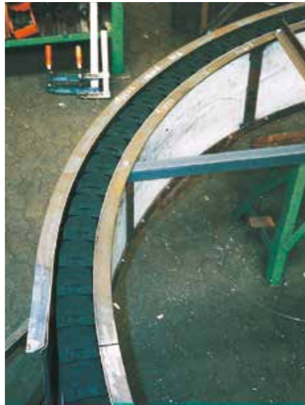
igus® system RM - guide troughs for circular movement applications with RBR
