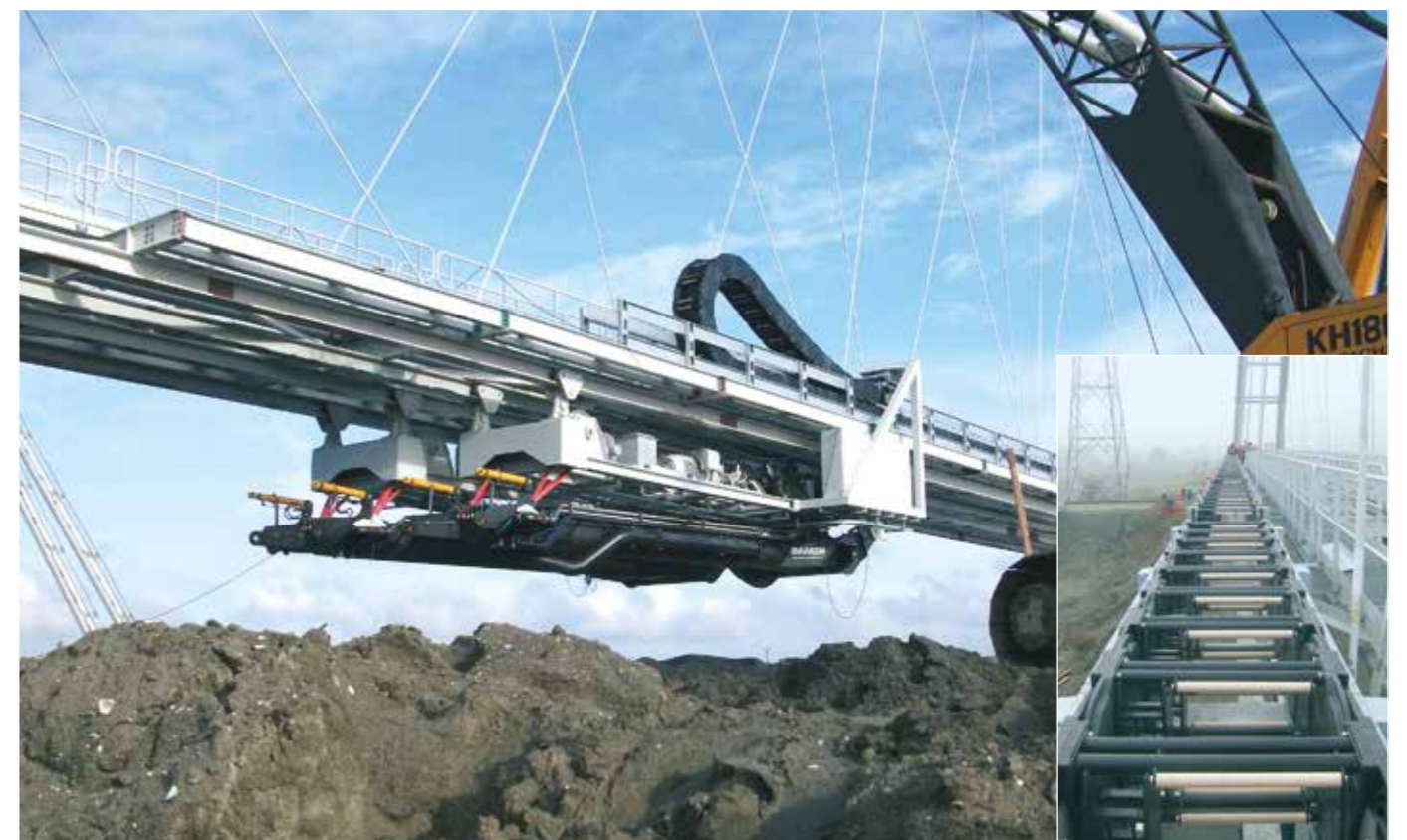
The world's largest polymer e-chain® with 350mm inner height: lighter than comparable steel chains, it effortlessly carries more than 100kg of fill weight per metre on a 138m travel
