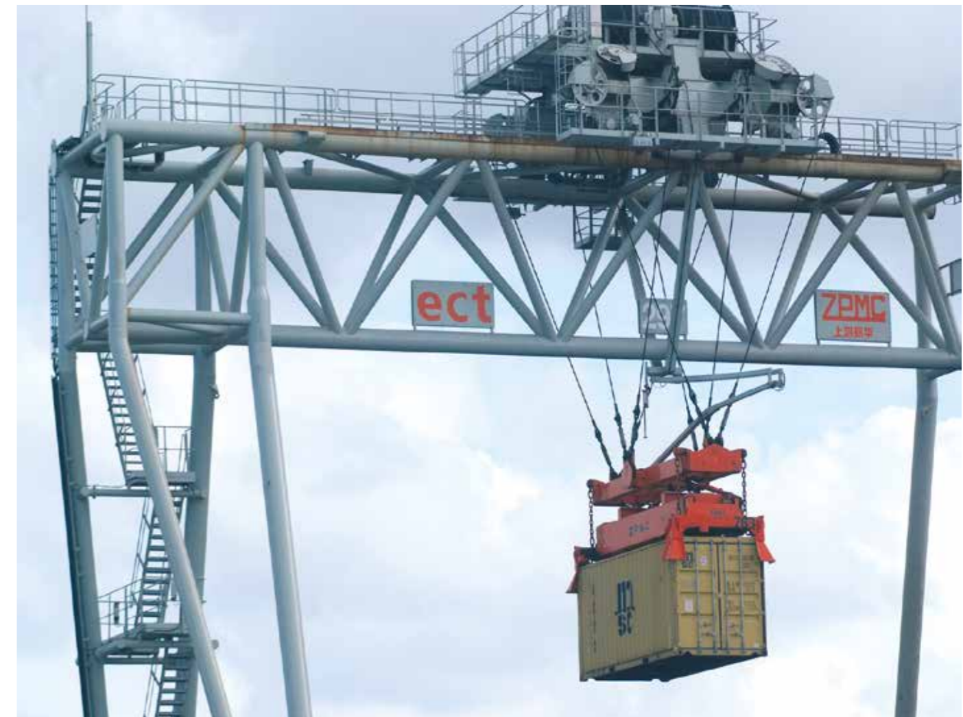
igus® E4/4HD e-chain system® on a container-crane. High loads and high speeds in difficult weather conditions
