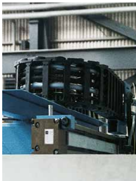
The lying e-chain®, one side of the igus® e-chain® is supported
