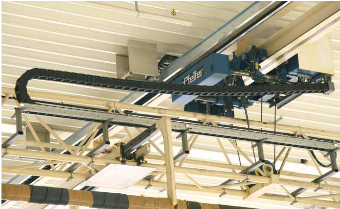
Handling unit indoor crane - long unsupported span with an igus® E4 series
