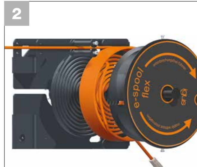
The e-spool® flex in detail from the inside (from left): housing, spiral guide, cables/hoses, winding housing
