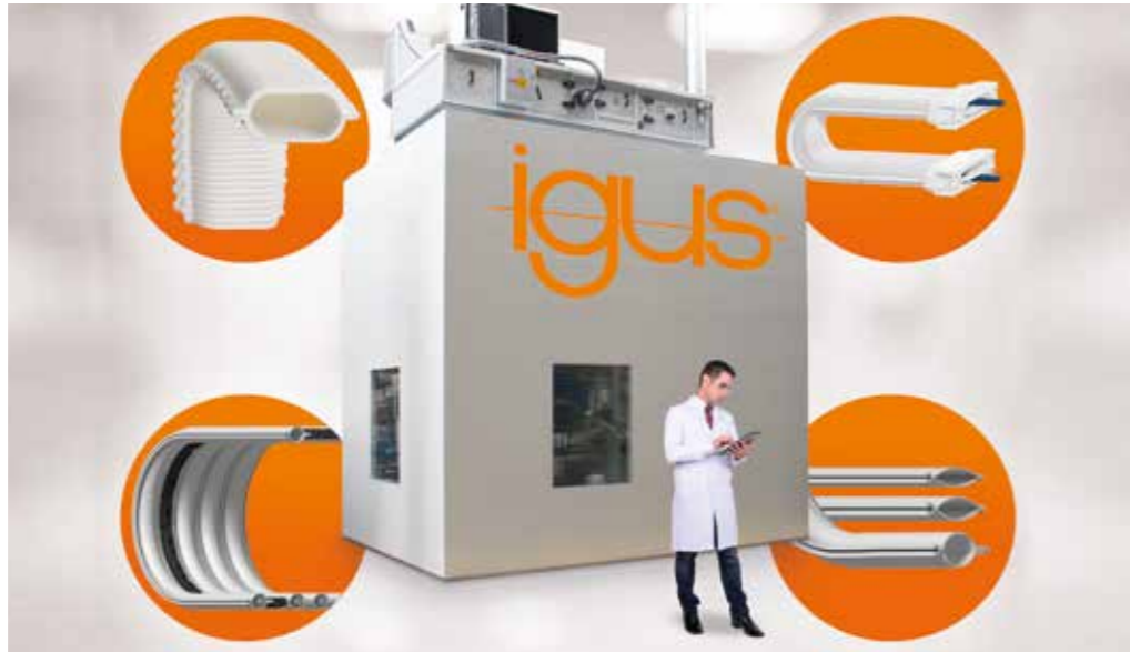
igus® cleanroom laboratory according to IPA certification ISO Class 1 in accordance with EN ISO 14644-1
