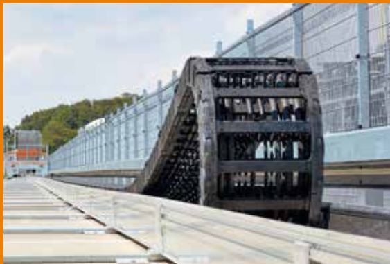
Outdoor test facility for travel lengths of up to 400m
