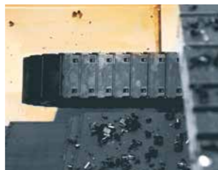
igus® e-tubes in the swarf area of a machine tool
