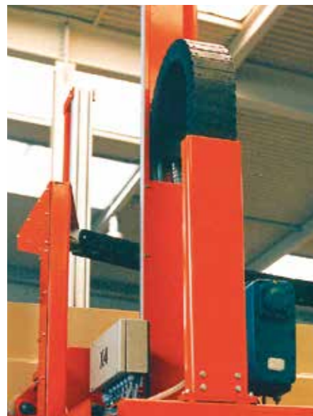
U-shaped supported igus® e-tube for high lateral acceleration
