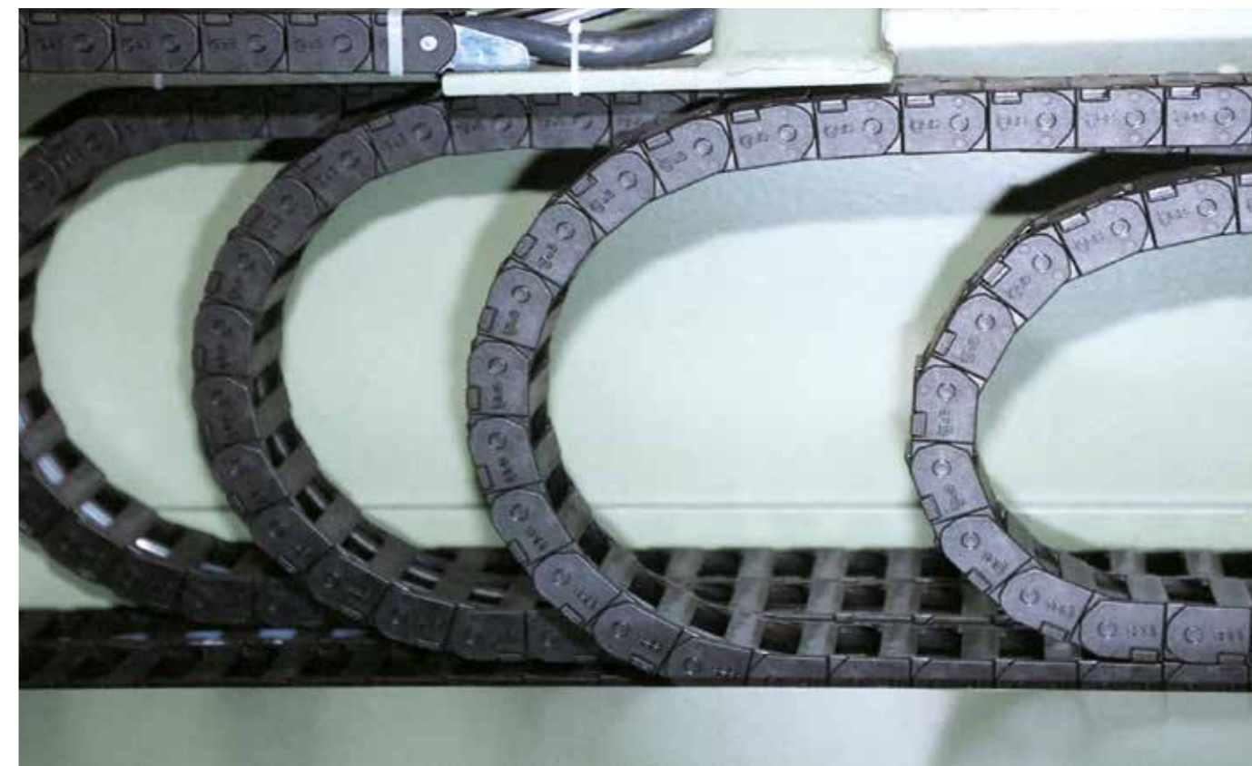
Five E2 mini chains installed above one another and side by side. The bend radii are exactly matched to each other
