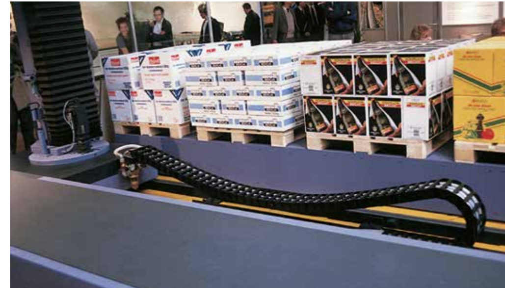
Example of unsupported with sag, FL_B
