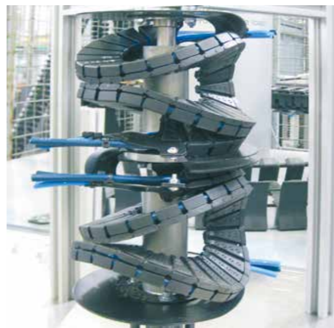
Two systems stacked above one another - this space-saving solution allows double filling space with a constant outer diameter of the system
