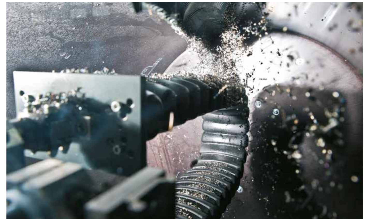
Swarf tests at the igus® test lab prove the excellent sealing of igus® RX e-tube. Video online ► www.igus.eu/RX_tested
