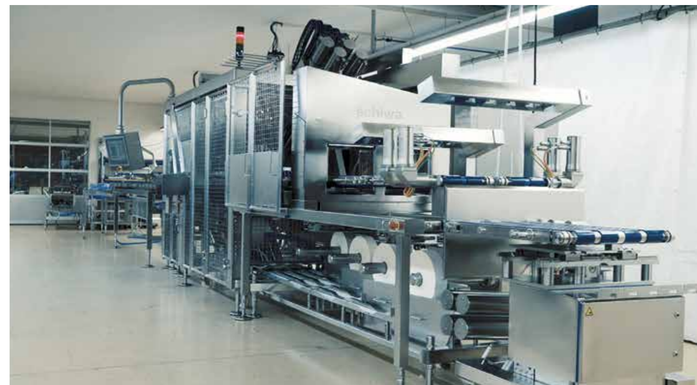
High-tech slicer complete line from Schiwa equipped with igus® RH3 e-chains® and four lead screws for slicing cheese
