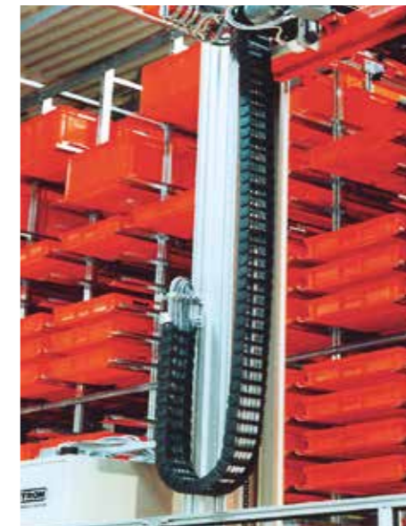
The E4.1 system is one of igus® best solutions for hanging applications
