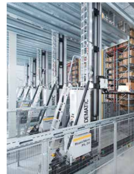
igus® guidelok slimline P vertical guidance in a high-bay warehouse, high reliability
