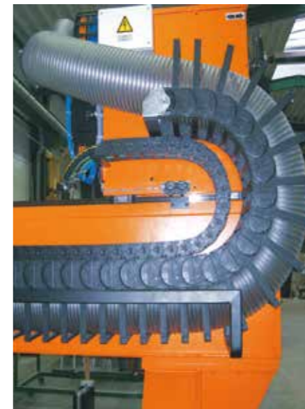
An E4 extender chain with vacuum hose also guides an E2 e-chain® here
