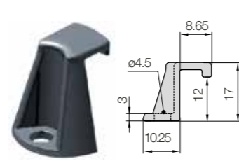
Part No. E3.10.00 Mounting angle as an individual part
