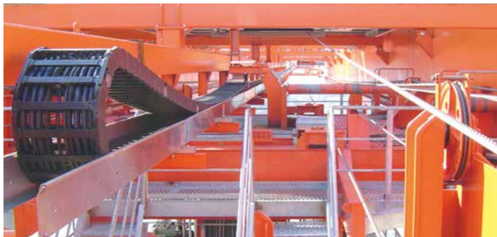
Long travel with an energy-efficient rol e-chain® - saving drive power
