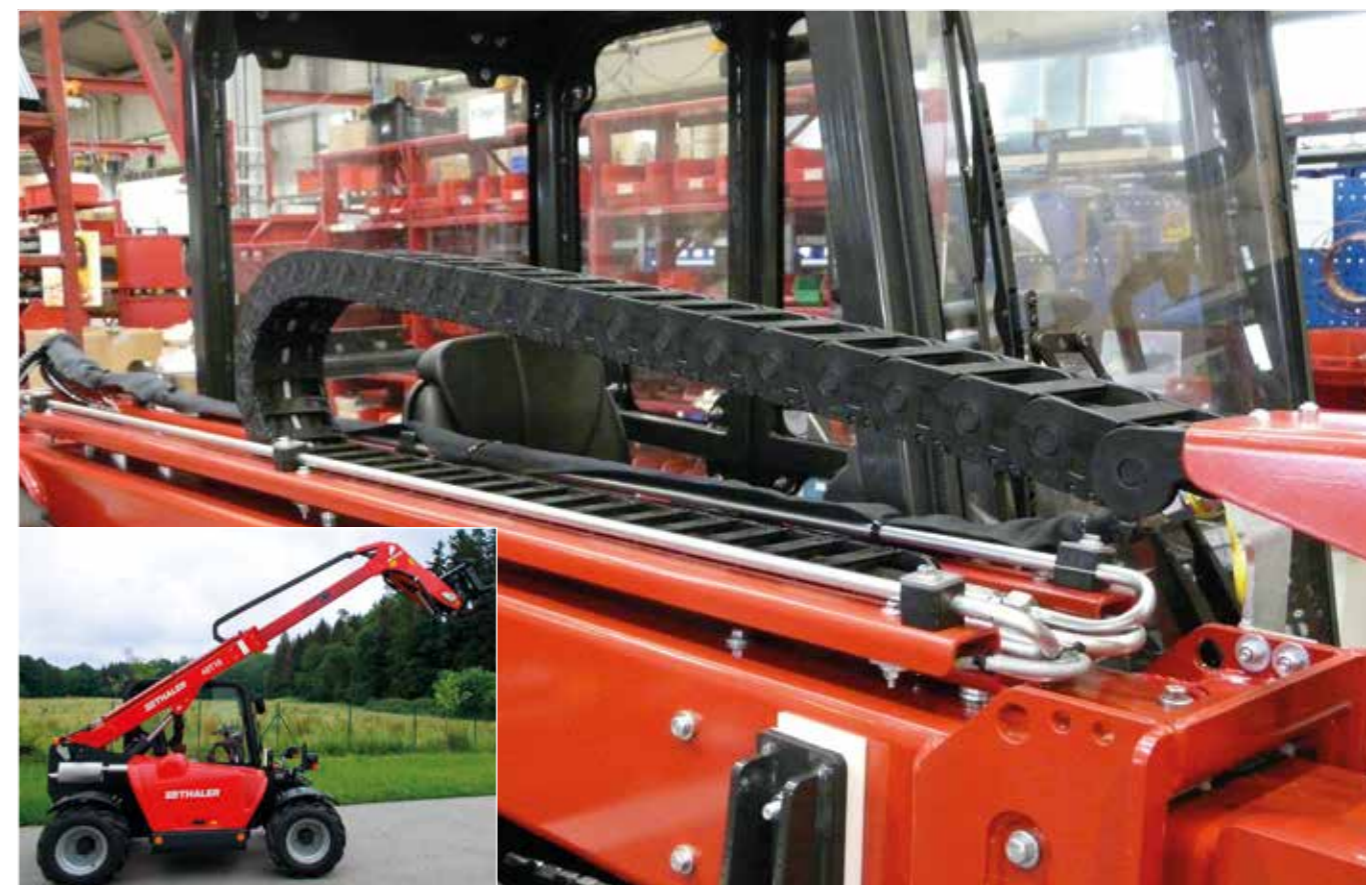
Telescopic loader - an E2/000 e-chain® guides the hydraulic hoses via the telescopic mast to the attachment
