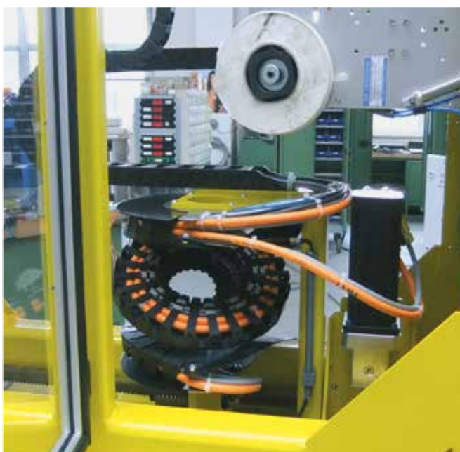
igus® twisterband TB30 for circular movements up to 360°, E2 mini and E2/000 e-chains® are used in this loading and unloading unit
