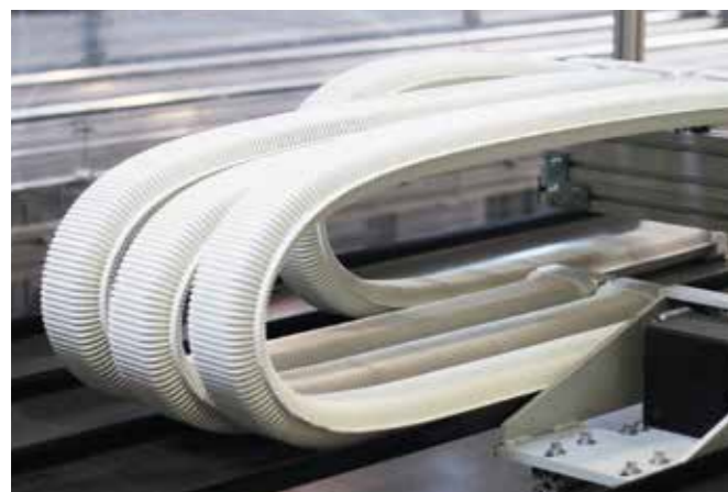
In the igus® laboratory, e-skin® withstood more than 10 million double strokes at 3m/s (issue 12/2020)
