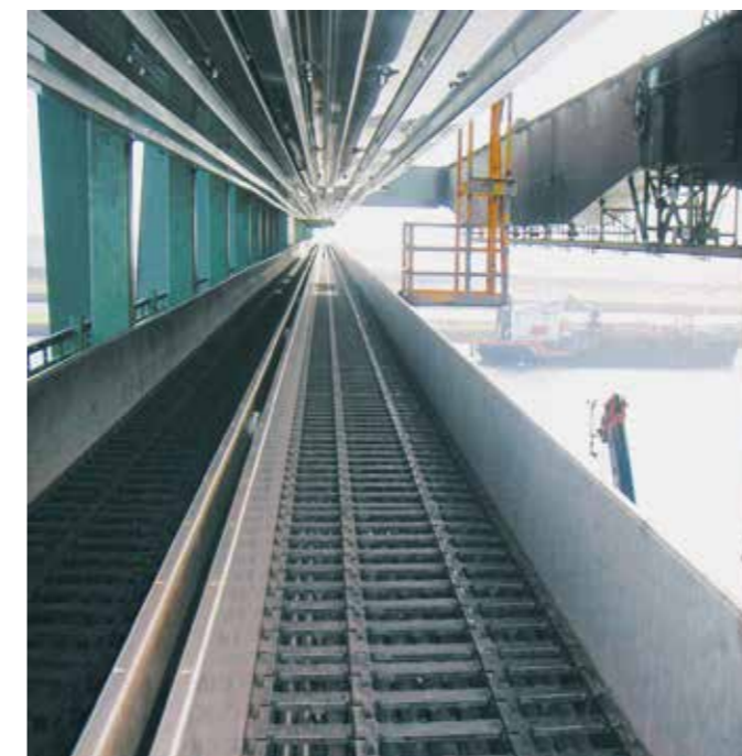
igus® system E4 with extension link on a ship loader for coal handling. Travel 105m, speed 240m/min, fill weight 53kg/m
