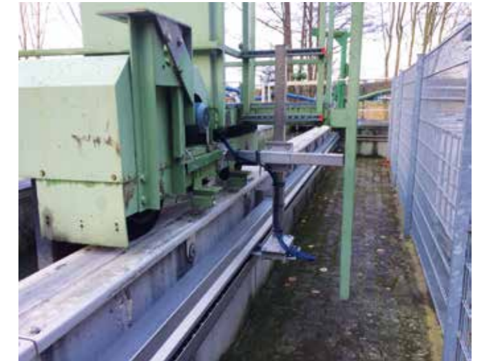
Sand trap with telescopic igus® moving end arm - travel 19m
