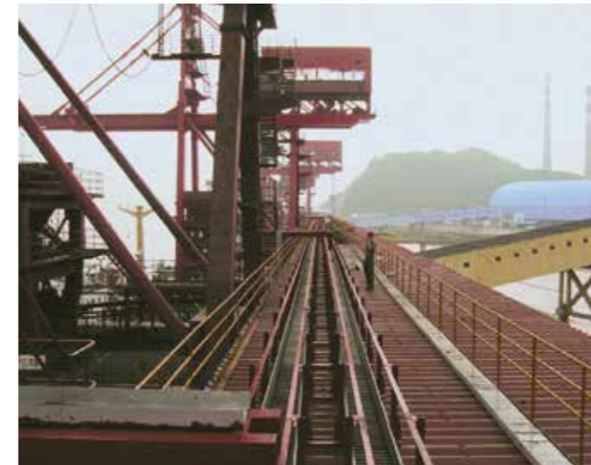
Series 4040R on a coal unloading system. Travel 190m, speed 0.5m/s, fill weight 8.05kg/m
