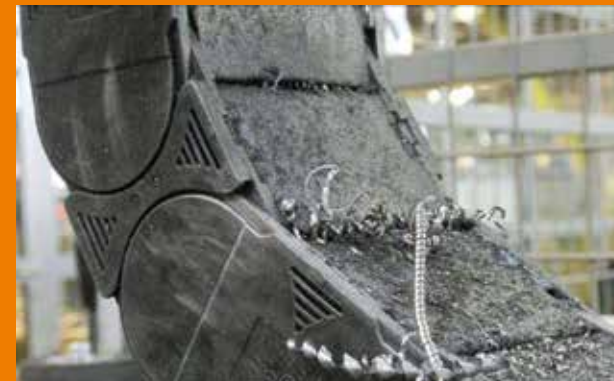
Swarf test, 100% swarf-resistant
