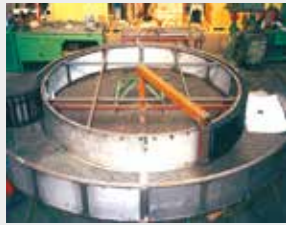
Circular movement with RBR , diameter 6000mm. The inner ring rotates
