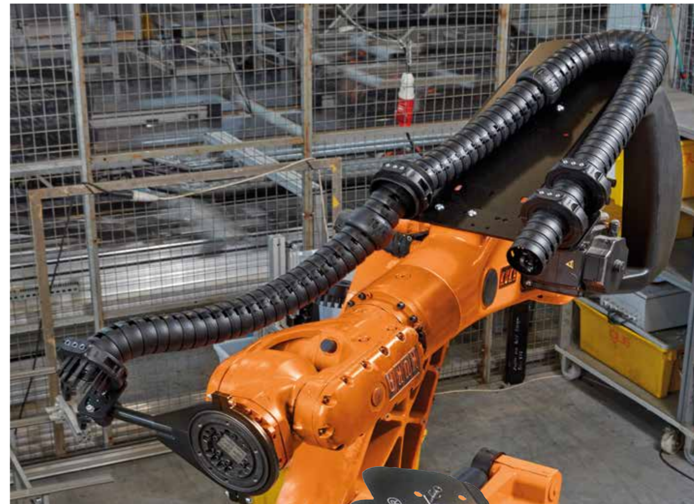
triflex® RS for a low profile retraction system. With triflex® RS, the multi-axis triflex® R e-chain® is routed parallel to the robot arm
