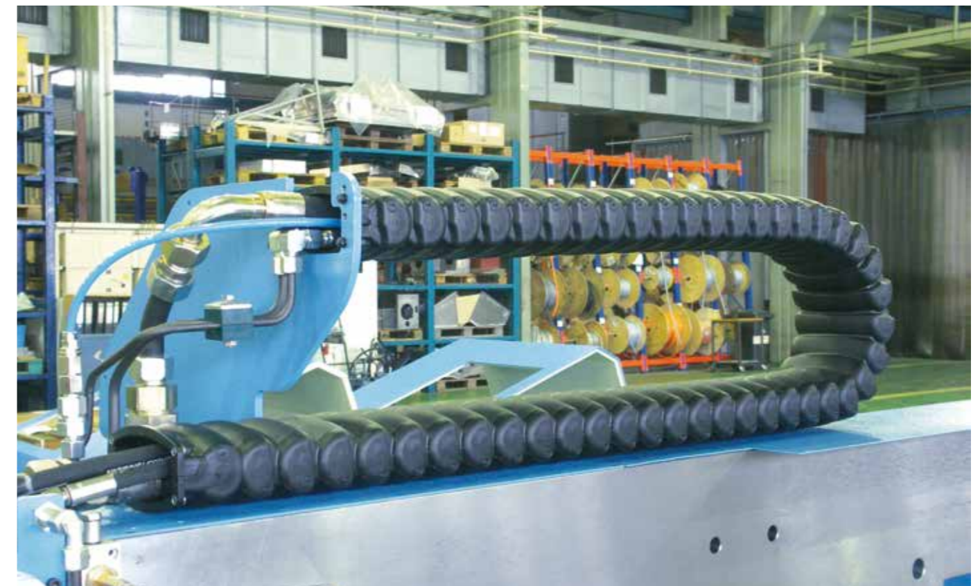
Supply of the main spindle in a tooling machine with igus® RX e-tube. The rounded contour of the energy supply repels all kinds of swarf
