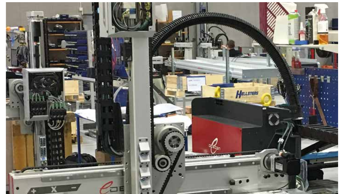
The igus® e-rib corrugated tube reinforcement can be easily retrofitted onto existing systems
