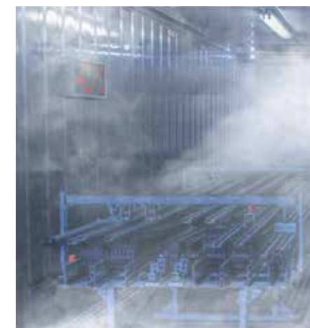
Tests in the igus® cold chamber are carried out under realistic real-world conditions with a moving e-chain
