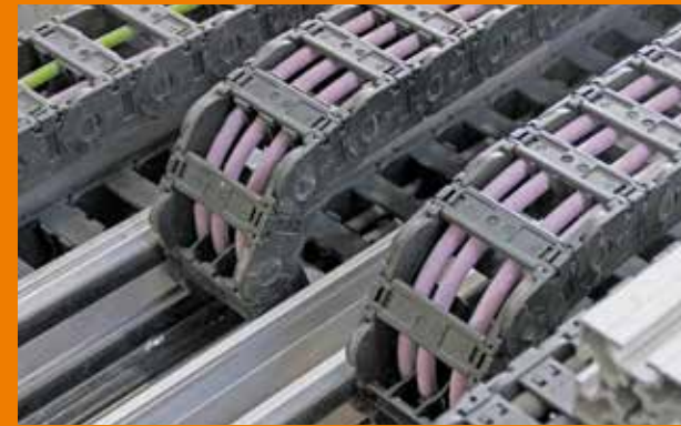
Cable test, more than 80 million strokes
