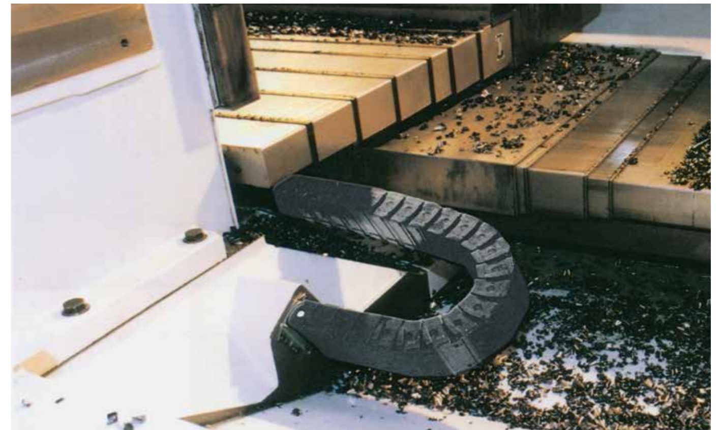
E2 e-tubes in swarf area of a machine tool. With igumid HT material resistant to swarf up to +850°C
