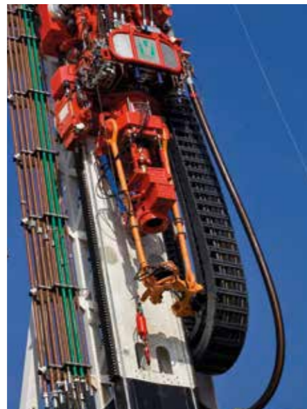
Hanging applications with heights over 100m are possible with e-chains®
