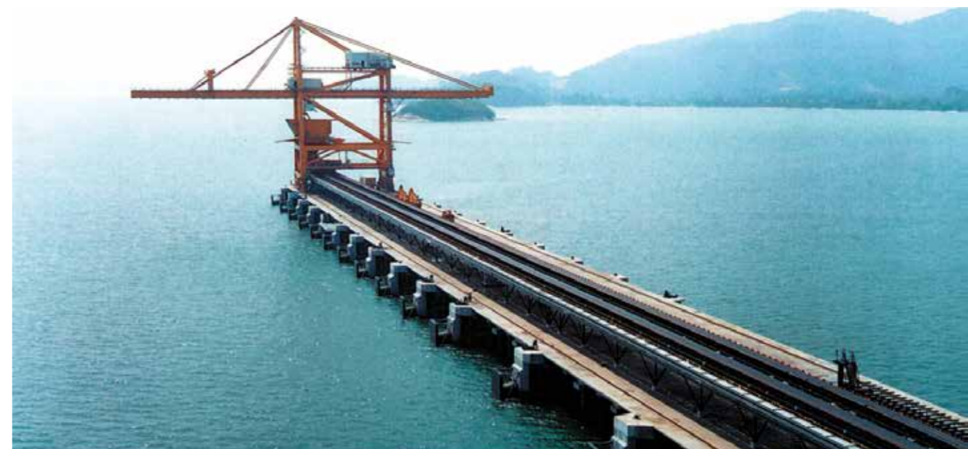
Cross travel of 441.3m, implemented with igus® E4/4 rol e-chain® series 5050R
