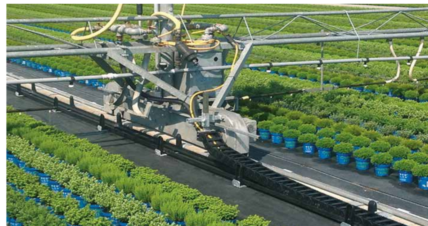
E2/000 rol e-chain® in a guidelite guide trough on an irrigation plant
