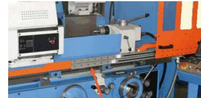
drylin® NT LM in guard door adjustment in a machine tool
