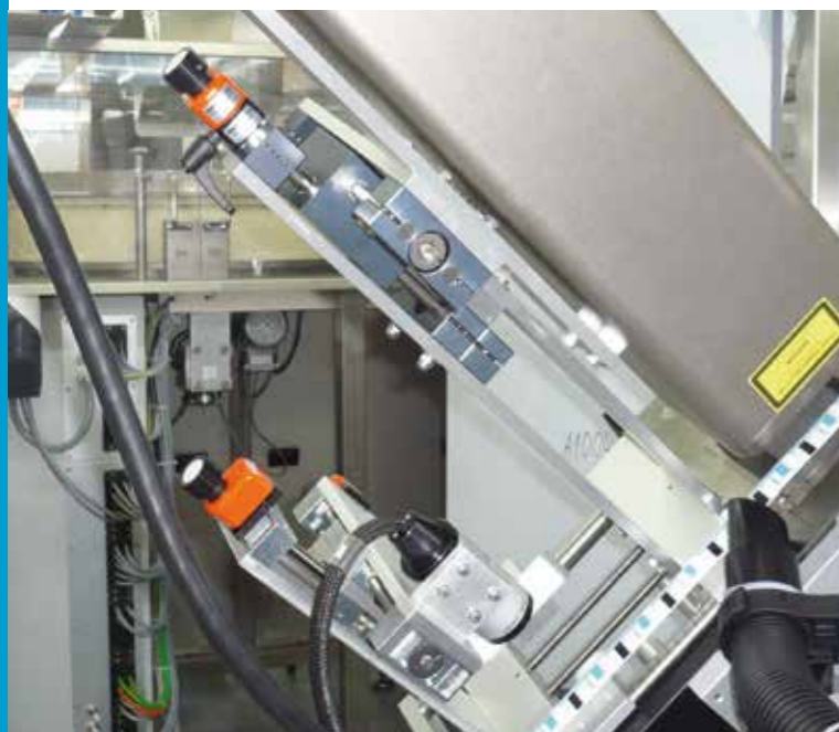
Camera/laser adjustment in labelling system In a labelling system the camera and laser positioning are guided with two drylin® SHT/SLWE-XY XY table units. (Fa. Pago Etikettiersysteme GmbH)
