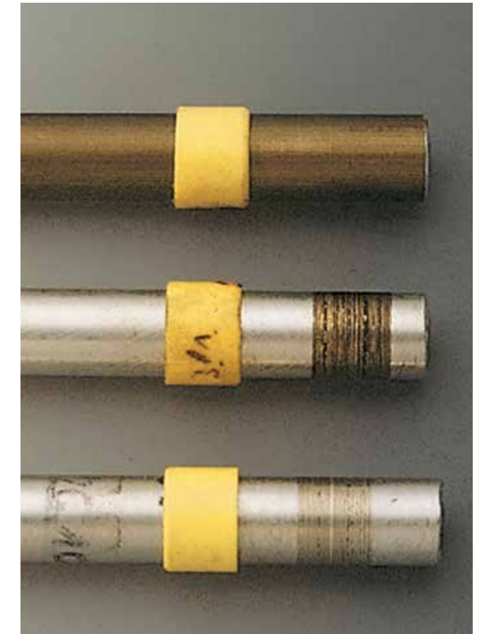
Picture 8: Wear experiments with aluminium shafts
