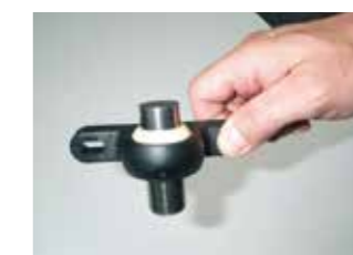
Tolerance test with plug gauge
