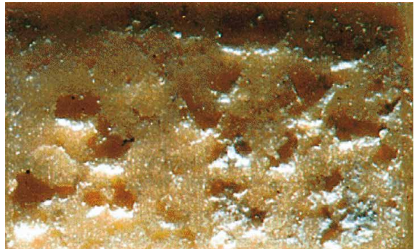
Picture 9: Erosion damage due to shafts that are too smooth
