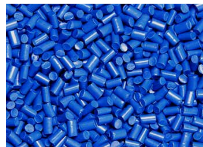
Picture 04: Polymer granulate; basis compound of the lubrication-free and predictable iglidur® plain bearings
