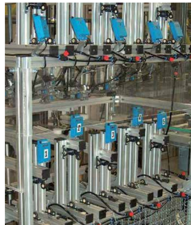
Picture 11: Pivoting wear test rig for testing the wear in pivoting movements at medium loads
