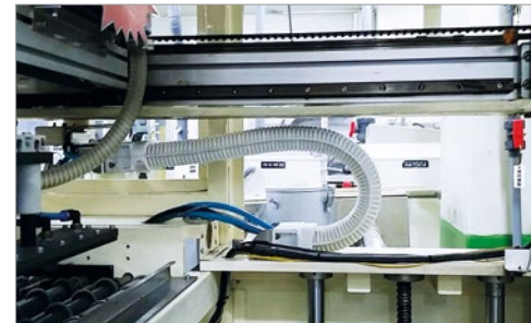
Absolutely dust-free environment for printed-circuit-board production using the abrasion-resistant e-skin®.
