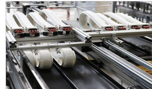
Service life test in the 3,800m² large igus® laboratory in Cologne (Germany).
