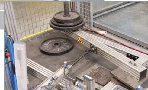
Load capacity of the locking system tested in the igus® test laboratory
