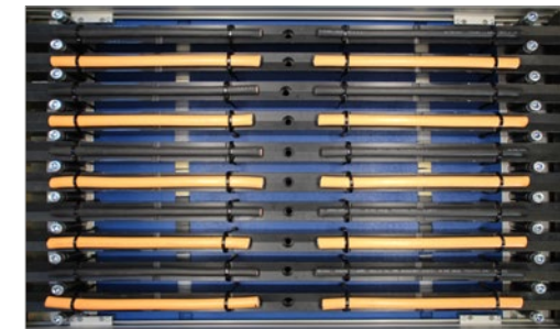
Tests in the igus® laboratory: various gliding combinations are tested and evaluated for abrasion.
