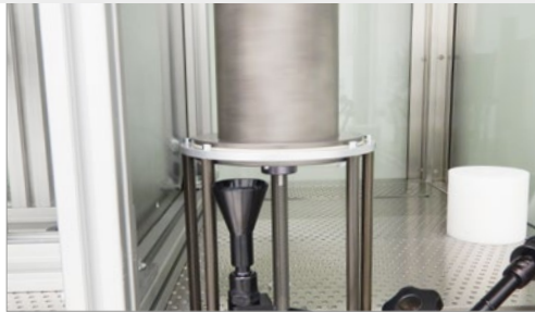
Particle emission test in IAF-compliant cleanroom laboratory
