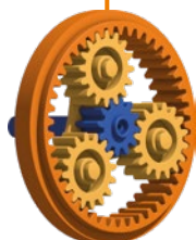
lubrication-free planetary gearbox
