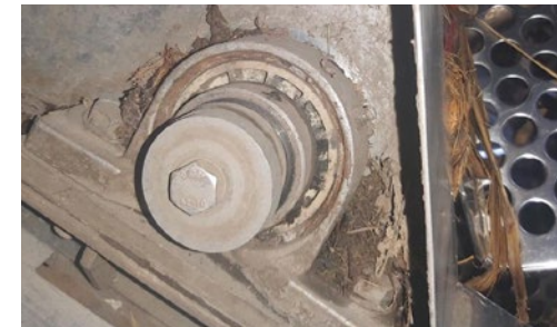
igubal® spherical insert bearing in injection-moulded design in a composting plant
