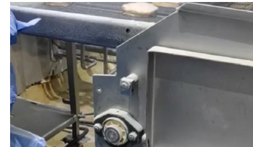
Polymer housing with injection-moulded igubal® spherical insert bearing in a conveyor belt for foodstuffs
