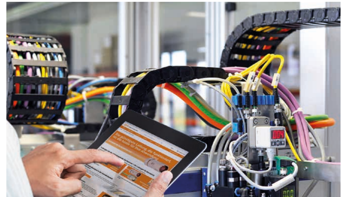
chainflex® CF888 bus cables in a handling application
