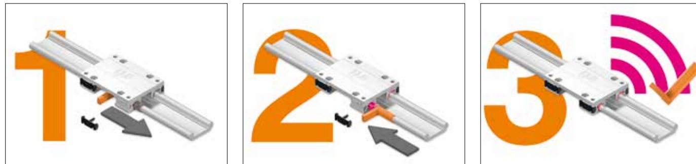
Simple bearing liner replacement.
