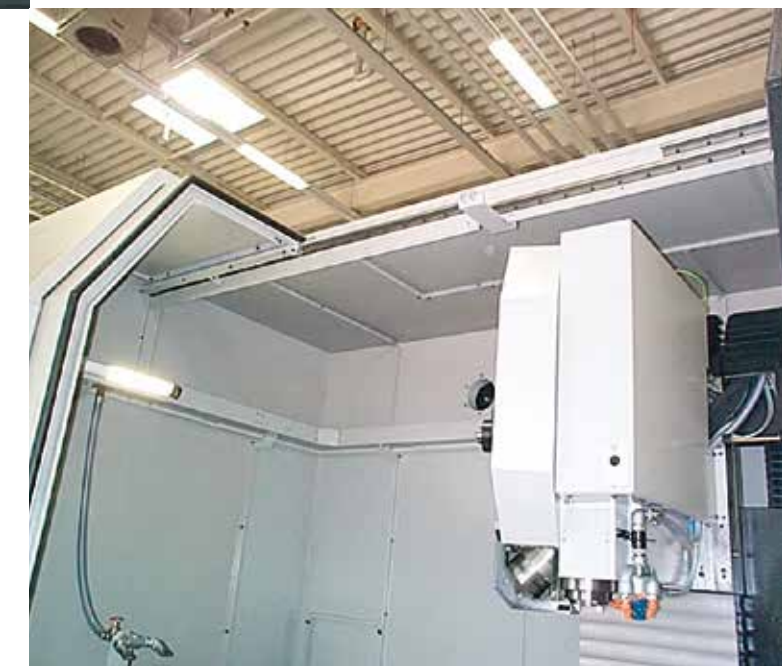
Door adjustment The smooth, quiet operation and the enormous cost advantages are obtained by the use of drylin® R linear plain bearings on the hard-anodised guide shafts to guide the doors of machine tools. (Alzmetall GmbH + Co. KG, Germany)
