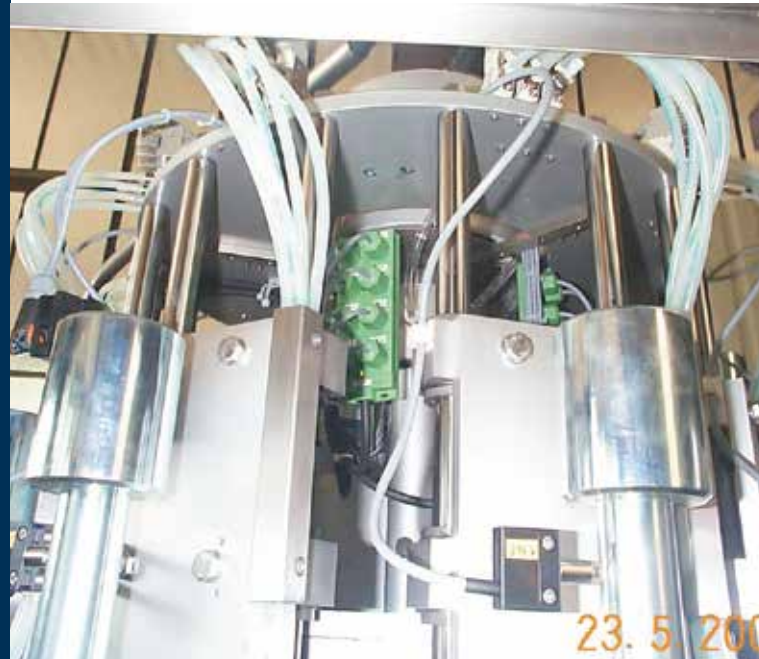
Champagne bottle sealing machine Due to freedom from lubricants and chemical resistance, drylin® guides score highly in facilities in the food sector. (Sick International Kellereimaschinen GmbH, Germany)
