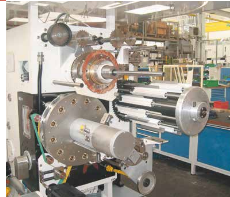
System for the production of aluminium cartridges The absolute freedom from lubricants and the resistance to prevailing paint mist led to the application of drylin® R linear plain bearings. (Mall + Herlan GmbH, Germany)
