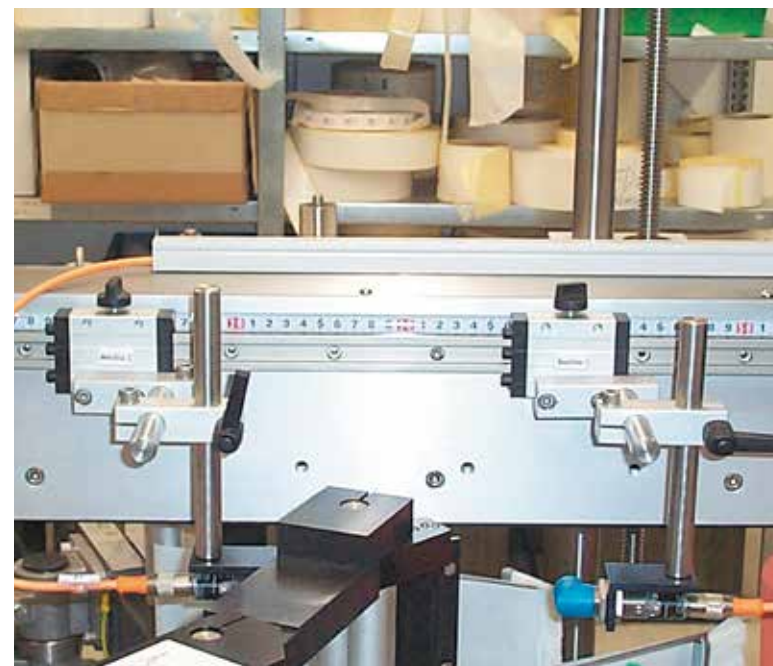
Label feeding system (packaging technology) Quick and flexible lubrication-free format adjustment at lower costs - implemented with drylin® T rail guide. Further advantage: guide carriage with manual clamp. (Geset Etikettier-Systeme GmbH, Germany)
