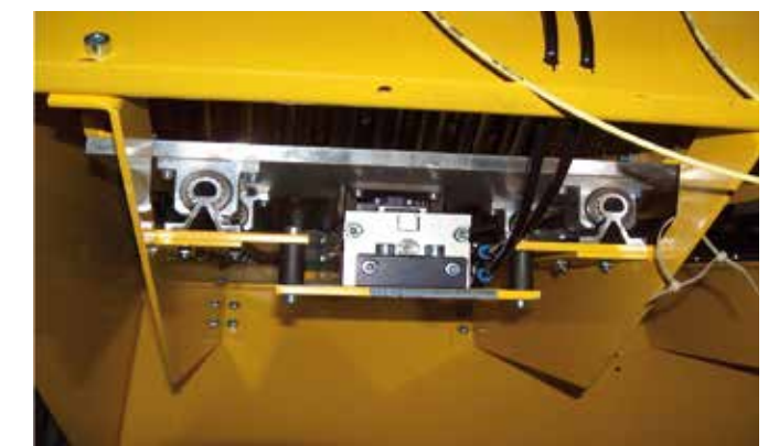
Cost-effective guide for work piece carriage in a machine tool with supported aluminium shaft.
