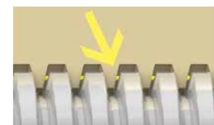
Yellow markings show the axial clearance of a standard lead screw nut
