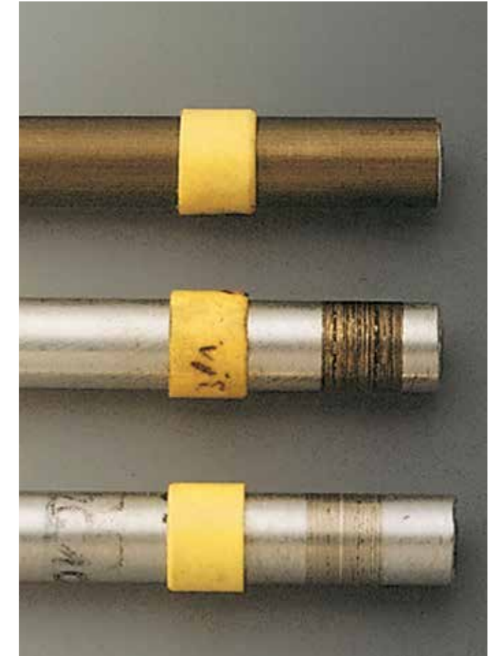
Picture 8: Wear experiments with aluminium shafts
