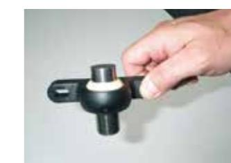
Tolerance test with plug gauge
