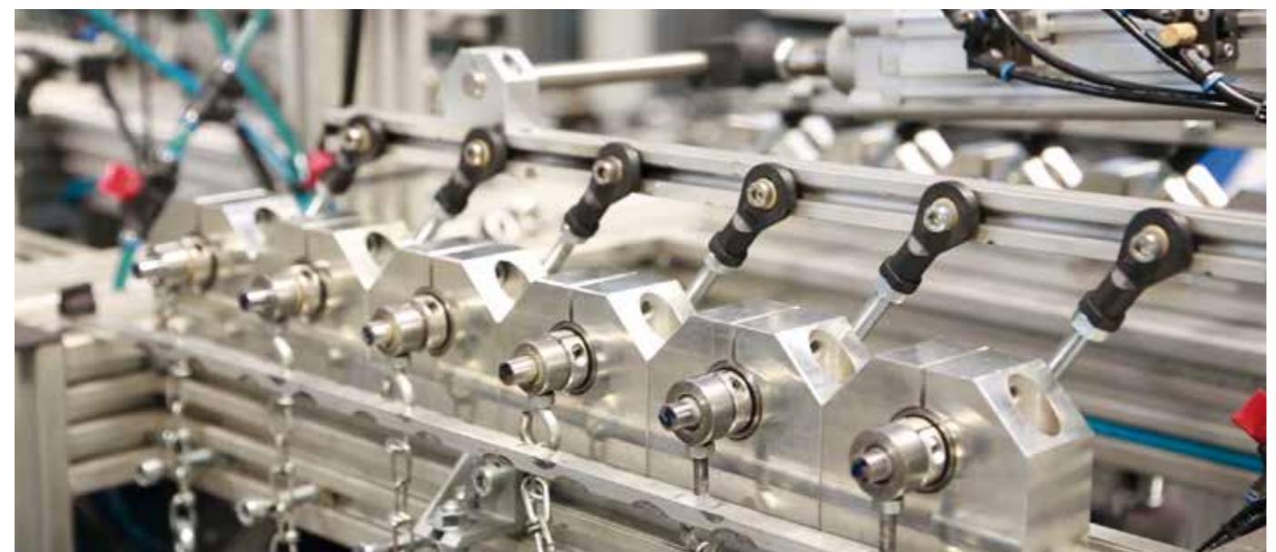
Picture 01: igus® test lab: More than 13,000 tribological tests (friction and wear) each year in 300 test rigs in the industry's largest laboratory (3,800m<sup>2</sup>). View inside igubal® test rigs.
