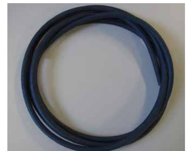
Result chainflex® TPE jacket: Cable after the 520,000 strokes test
