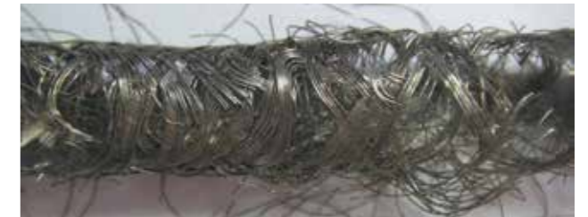
The detail inspection of the shield braid shows damage on the shield strand wires.
