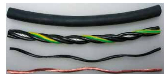
The individual elements of the CF9 from the dissected cable.
