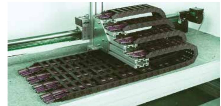
Example at igus® test laboratory: constant development and testing of chainflex® cables
