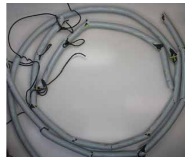
Result PUR jacket: Broken after 41,000 strokes
