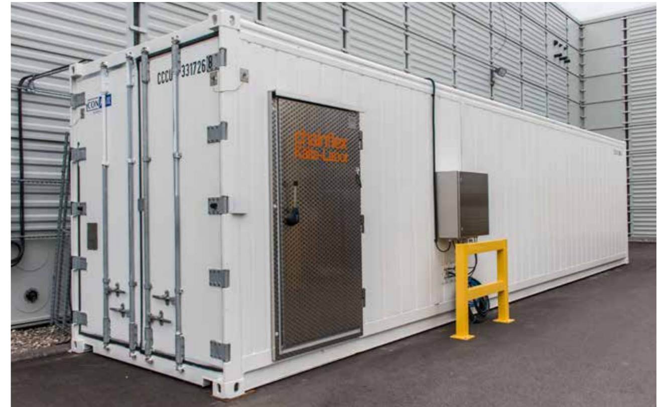
40-foot climatic container for cable tests in continuous motion at -40°C
