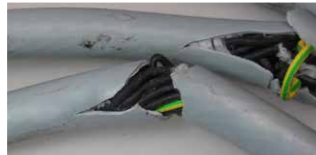
Jacket damage after 41,000 strokes ...
