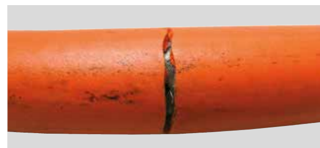
Cracks in the outer jackets of materials from competitors caused by the use in e-chains®.
