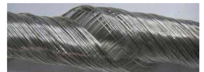
Picture 3: Detail pictures of the CFROBOT after more than 3 million movements of \pm 270^\circ
