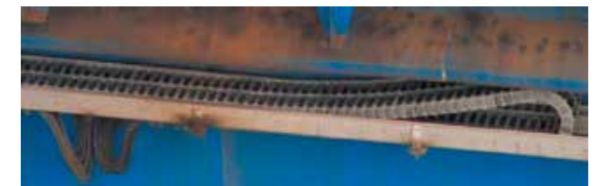
An igus® energy supply system with a length of approx. 26m in a stainless steel trough.
