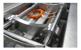
GEA uses xiros F180 plastic ball bearings in the film guide rollers of its thermoforming packaging systems. The maintenancefree automatic web edge control with drylin trapezoidal lead screw nut and drylin R liners creates the conditions for processing various film qualities.
